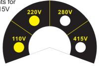
The Voltage Detector with LED: The led Voltage Detector lit up as soon as there is enough voltage across the tips between the poles. This indicates that voltage between the tips has reached a dangerous level and therefore could be lethal. Once the Led lit, be extra careful.
