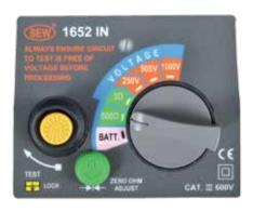
Always check for voltage before testing and measuring on a circuit. This instrument is intended for measuring Low  $\Omega$  and Insulation resistance on unenergized circuits only. Use the procedure explained at points 9.2, 9.3, 9.4.
