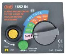
Turn the function selector to Batt. Check. This function has a load which draw about 205mA when test is performed, and therefore it is doing a worst case battery test.
