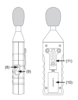
(8) Output: AC output 1 Vrms for full scale (50dB).
