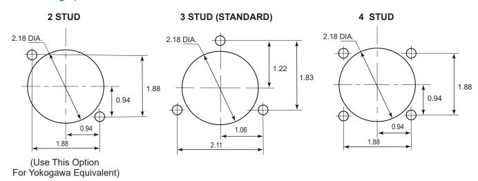
The mounting studs on the 5000 Series can be ordered to fit your existing panel openings at no extra cost.
