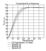
A low range AC voltmeter offering a performance close to that of a full specification VU meter. Suitable for connecting across a  $600\Omega$  line and self contained except for requiring an external 3k6 resistor. Calibrated for use with a 3k6 ohm resistor 4vu above the scale marking so that the reference deflection (0vu) is produced by a signal 4vu above 1mW in  $600\Omega(1.228V)$ .
