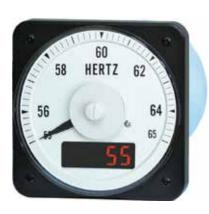
HLS-110DI TWO-VUE switchboard meters are combination Digital / Analog indicating instruments. They can be configured to accept VAC, AAC, VDC, or ADC input. Both the digital and analog displays can be modified to represent virtually any scaling or engineering units as
