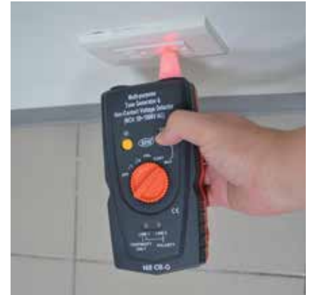
Detect voltage in wall outlet
