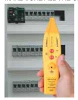
Now, for example, start scanning from the top left row, then go down etc..., But you can scan the breakers in any order. While you are scanning, observe the bar-graph and listen to the buzzer.
