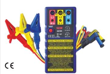
The 888 PMR is a 3-Phase Presence and Rotation Indicator combined with a 3-Phase Motor Rotation Tester. It can be utilized on either a powered system (the supply side) or an unpowered motor (the load side) with no damage to the tester.
