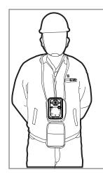
Please remember to put the 302 SVD into the soft pouch before doing the voltage detection. Put the safety voltage detector on your chest with the shoulder belt around your neck.
